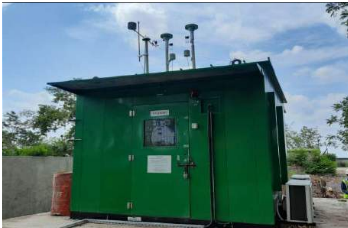
CAAQMS -01 installed at Plant Main Gate
