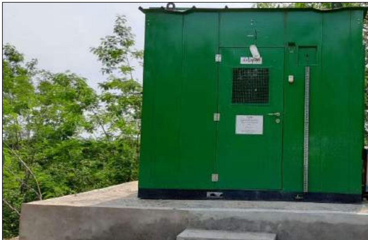
CAAQMS -03 Installed at Crusher Area (Mines)
