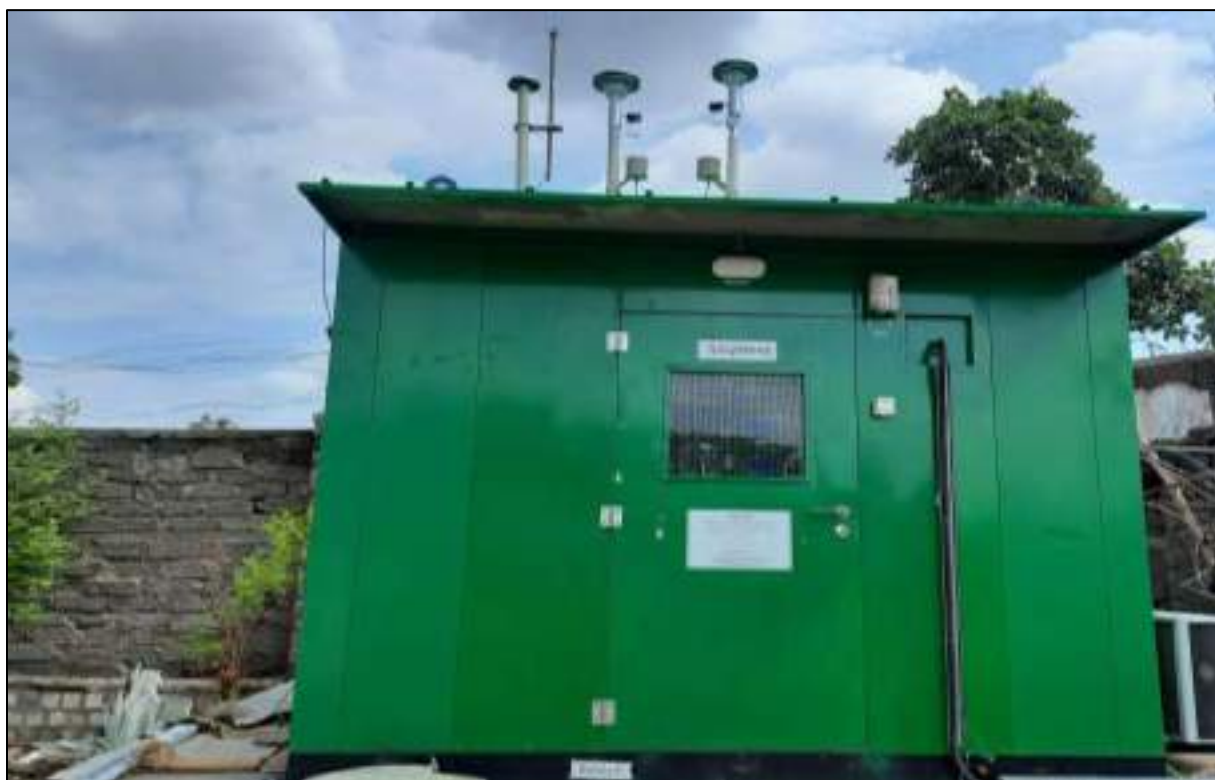
CAAQMS -02 installed at CPP Area
